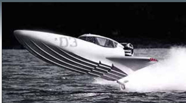
An outboard-powered XB-23, a test boat, launches off a wave in 2004. Note the winglets, and a canopy that safeguards life and limb. Racing in the UIM 2-Liter class, the 24.3' x 9.8' (7.4m x 3m) boat did 75 knots with 220 hp (164 kW).
